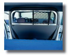
with roll bar style 1 5/8 inch structural tubing and padded with 1/2 inch foam. -Easy No-Holes drilled and no trim
